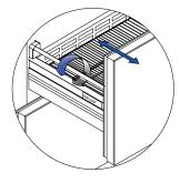
Vertical adjustment of the front. Make sure that the magnetic gasket seals adequately
